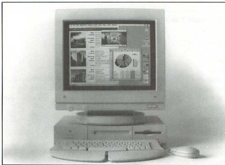
Figure G.15 The Quadra 610 is a low-cost Macintosh that includes built-in Ethernet.
